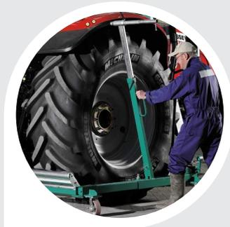
Capable of handling large wheels from 1250 mm up to 2400 mm in diameter and up to 1050 mm in width.
